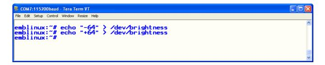
• 2. Step: The E2POT driver within the eSOM/2586 Linux O/S is controlled by integer numbers between 0 and +64. 0 stands for backlight (full) off. +64 turns the backlight full on. Any number between 0 and +64 dims the backlight. Please try the following command sequence and watch the LCD backlight:
