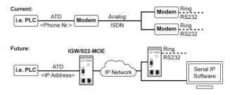
Replacing analog modems with the IGW/922-MOE
