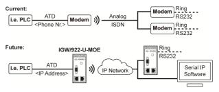
Replacing analog modems with the IGW/922-U-MOE
